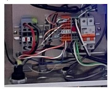
Figure 2-5 – SC 372 Flashhead Cable Connection
