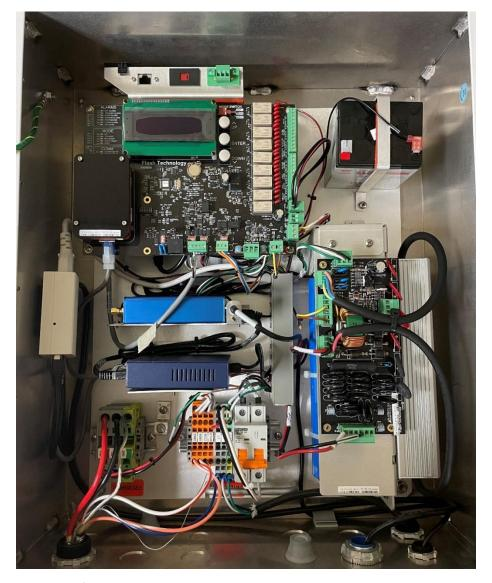
Note: Shows a fully loaded unit with optional modem, Wi-Fi and generator monitoring kits.
