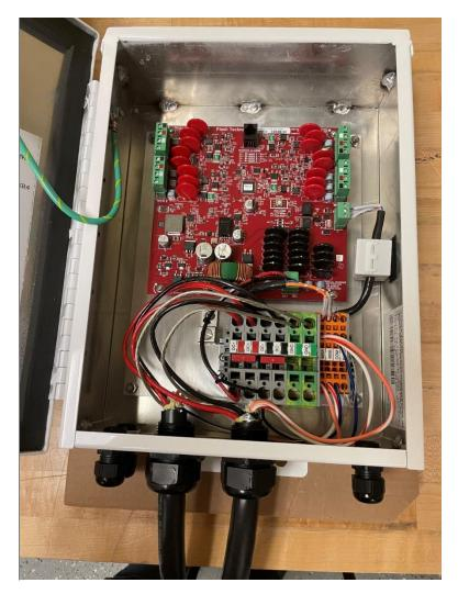
Figure 2-6 - Marker Interface Box and Wiring
