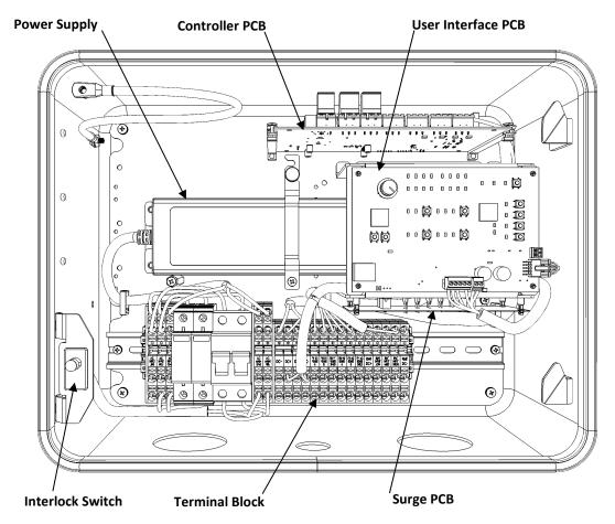
Figure 1.2 - PC 800(L) Internal Components
