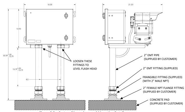
Figure 2.2 – System Dimensions and Mounting Details
