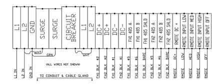
Figure 2.3 - System Input Wiring
