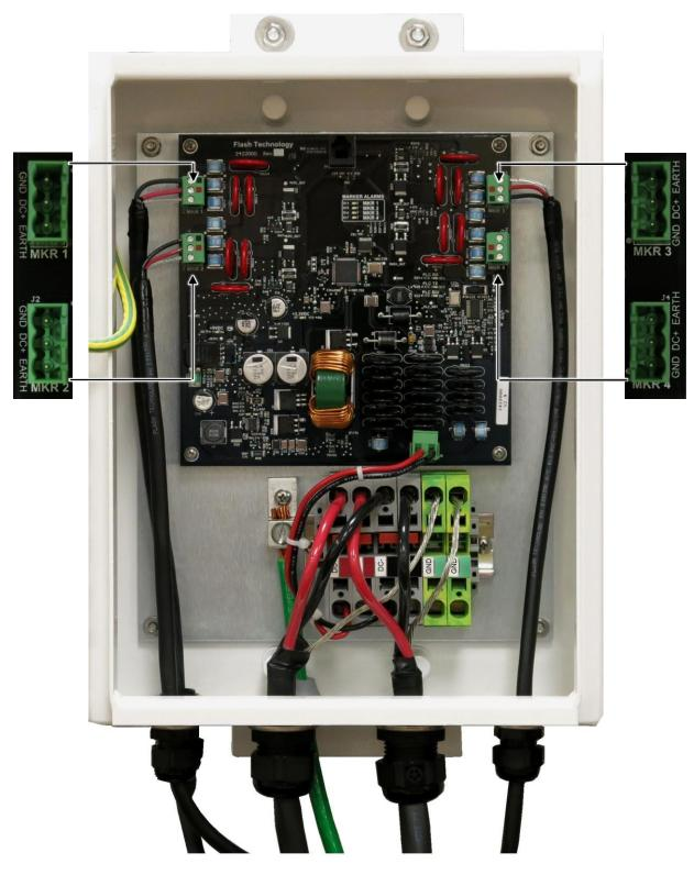
Figure 2-6 – Marker Interface Wiring
