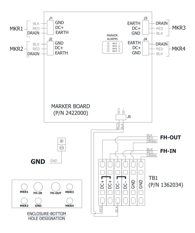
Figure 2-32 – Marker Interface Enclosure Wiring Diagram
