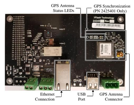
Figure 1-5 – PCB 3 with GPS
