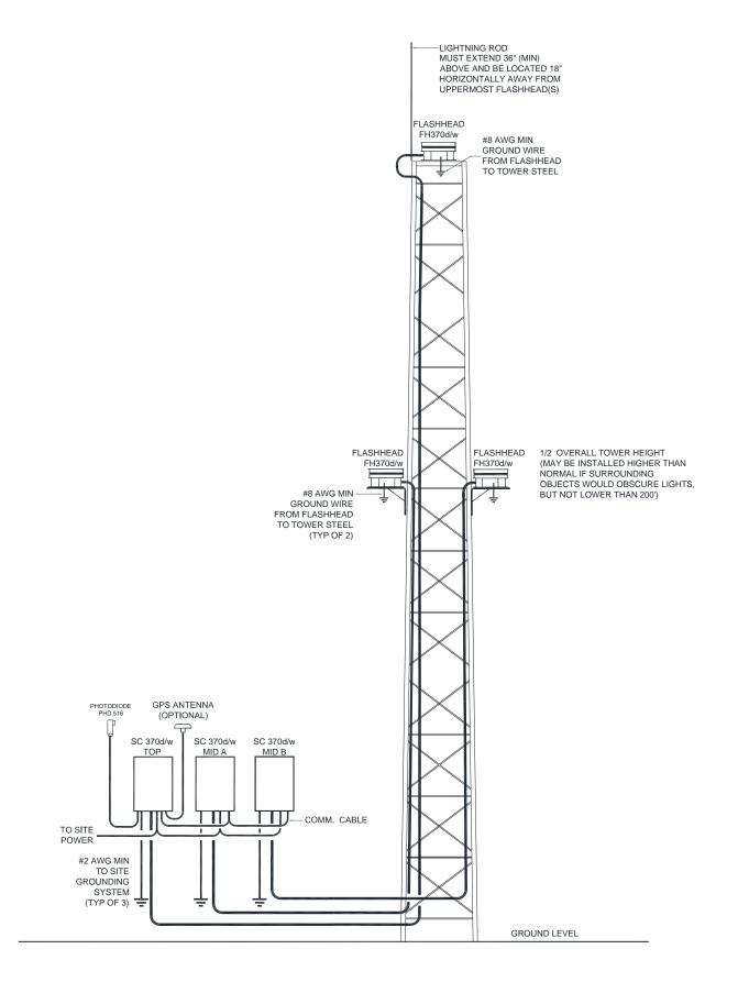
Figure 2-19 – Typical E2/D2 Avian Component Locations (AC 70/7460-1L)
