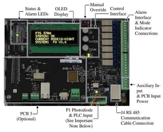
Figure 1-2 – PCB1 Controller Board
