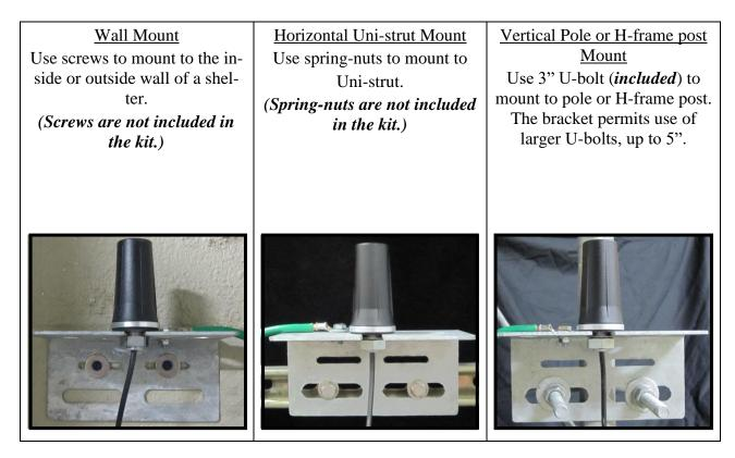
Figure 2-2 – Antenna Mounting Options
