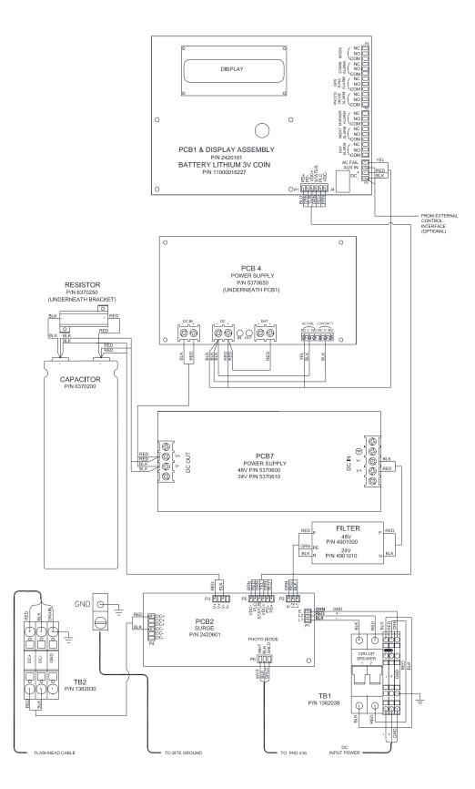
Figure 2-29 – SC 370 (DC) Internal Wiring Standard System
