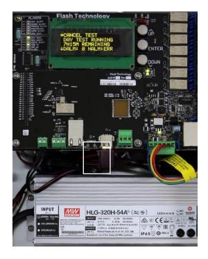
Figure 2-4 – USB Wi-Fi Installation
