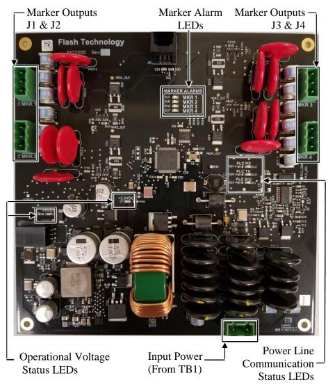
Figure 1-8 – Marker Interface PCB
