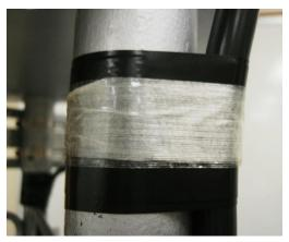
3. Wrap four full turns of two-inch Scotchrap #50 tape, or the equivalent, over the Scotchrap Filament #890 tape.
