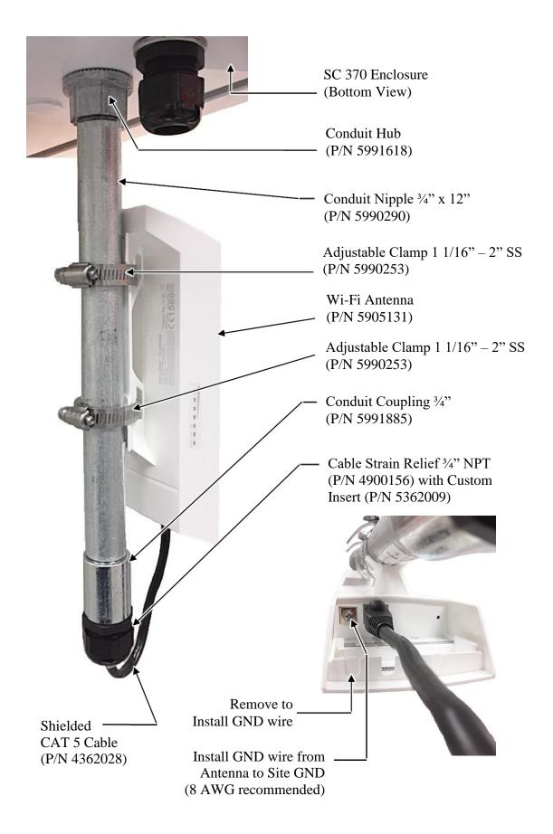
Figure 2-3 – Wi-Fi Antenna Installation
