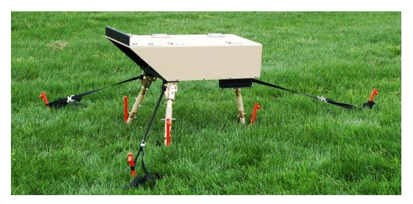
Fully secured LHA with ground stakes and straps
