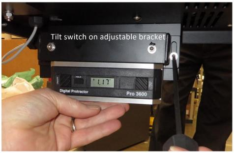
Tilt switch bracket detail
