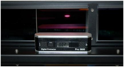
LHA with the digital inclinometer in place
