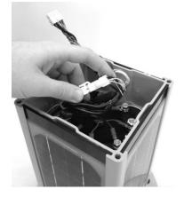
7. Reconnect the battery harness and press together until it is latched.
