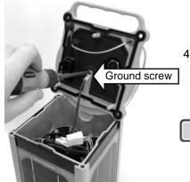
4. Using a #2 Phillips screwdriver, remove the ground screw from the top of the head. This screw can be recycled since it will no longer be used with the new head.
