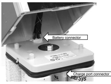
4. Using a 1/2 in. hex socket, remove the central bolt and its hardware
