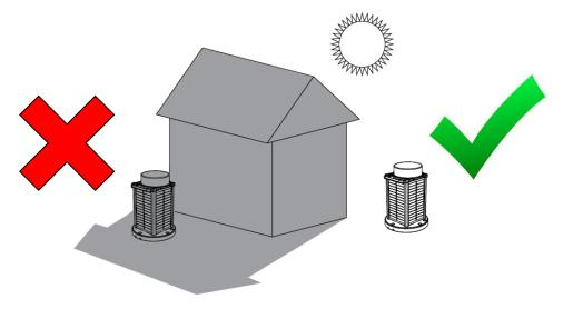
**Cooler is better:** The battery lasts longest if you can minimize its exposure to high temperatures. Choose a location that is away from hot, dark colored surfaces like asphalt or black steel plate. Mounting kits are available that elevate the light and can help reduce the temperature of the battery.
