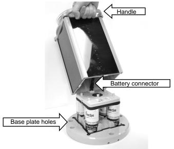
7. Tighten four base plate screws to 40 in.-lbs.
