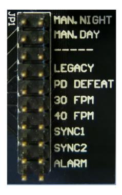
Figure 3-2 – Configuration Jumpers
