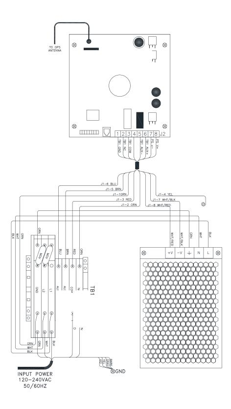
Figure 4-2 – Beacon Wiring Diagram (10 Conductor Option)
