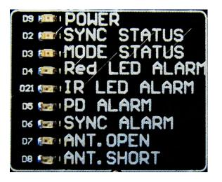
Figure 3-1 – Status Indicator LEDs
