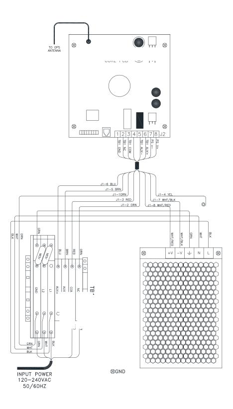
Figure 4-1 – Beacon Wiring Diagram (Standard)
