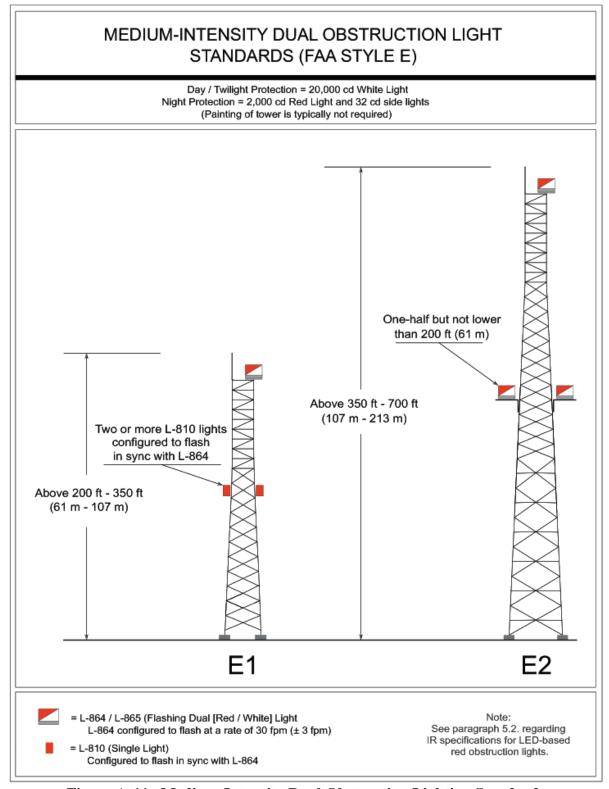
Figure A-11. Medium-Intensity Dual Obstruction Lighting Standards
