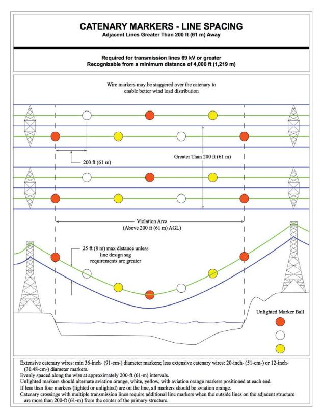
Figure A-3. Catenary Markers - Line Spacing (Adjacent Lines Greater Than 200 ft (61 m)
