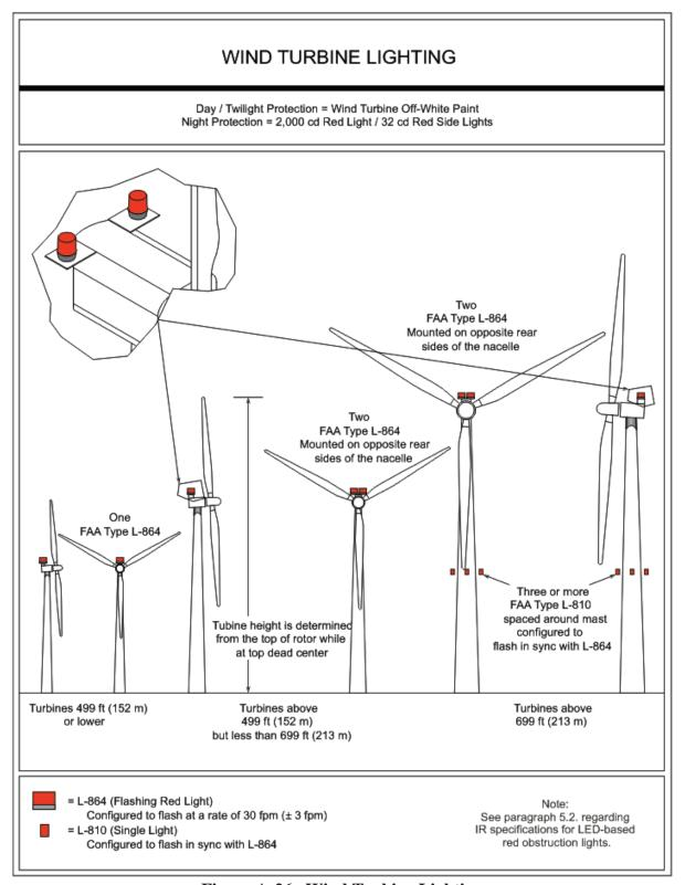
Figure A-26. Wind Turbine Lighting
