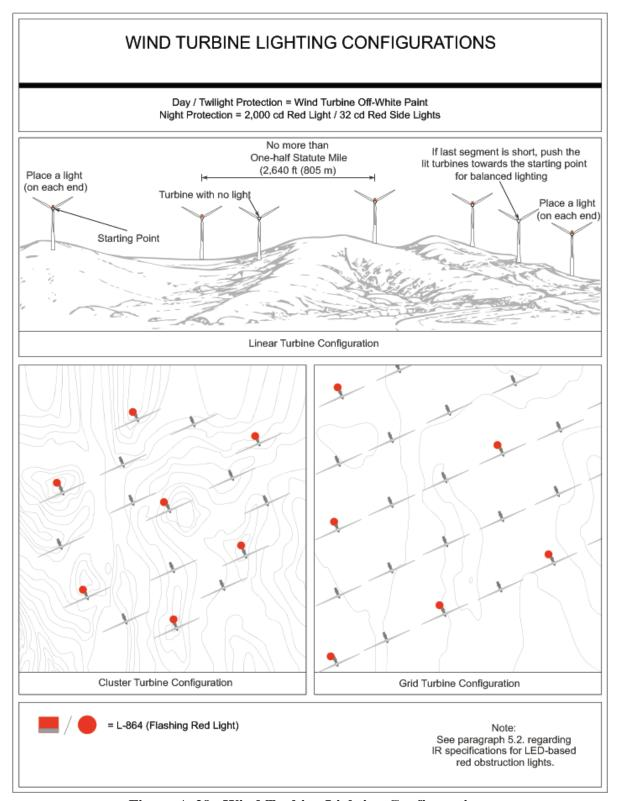
Figure A-29. Wind Turbine Lighting Configurations
