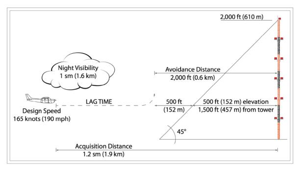
**Note:** The 2,000-foot avoidance distance comes from the guy wires of a 2,000-foot structure. The guy wires at a 45-degree angle would be at a distance of 1,500 feet from the structure at a 500-foot elevation. Since the aircraft is to be 500 feet clear of obstacles (the guy wire), the distance of avoidance from the structure is 1,500 + 500 = 2,000 feet. (See Figure B-1.)
