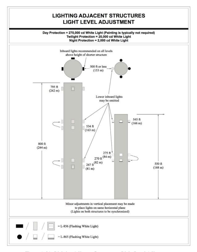
Figure A-21. Lighting Adjacent Structures—Light Level Adjustment
