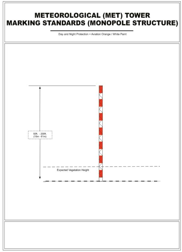
Figure A-16. Meteorological (MET) Tower Marking Standards (Monopole Structure)
