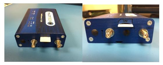
1.1.3 Ensure that the antenna is connected to the port marked "Cell" and not to the port marked "Aux".
