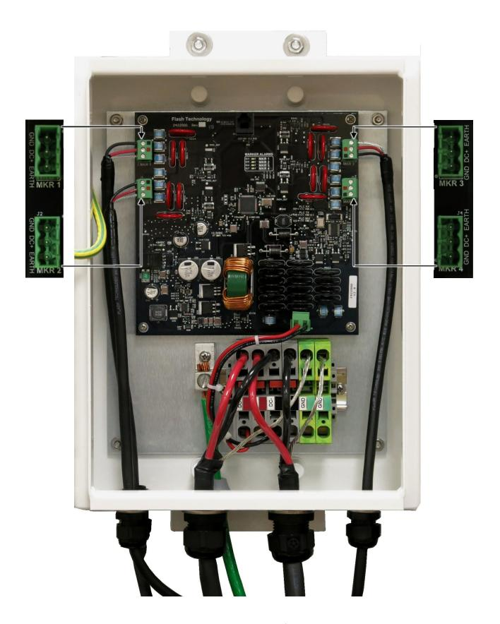
Figure 2-6 – Marker Interface Wiring
