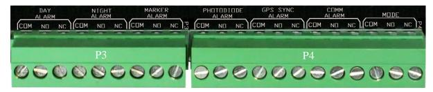
Figure 1-4 – Alarm Interface & Mode Indicator Connections
