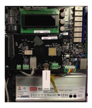
Figure 2-4 – USB Wi-Fi Installation
