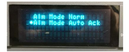
To change, use the Up button to move the arrow to the first option of "**Alm Mode Norm**".
