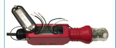
3. Using the supplied wire nuts and electrical tape connect the (2) Black wires, the (2) White wires, and the (2) Green wires together.
