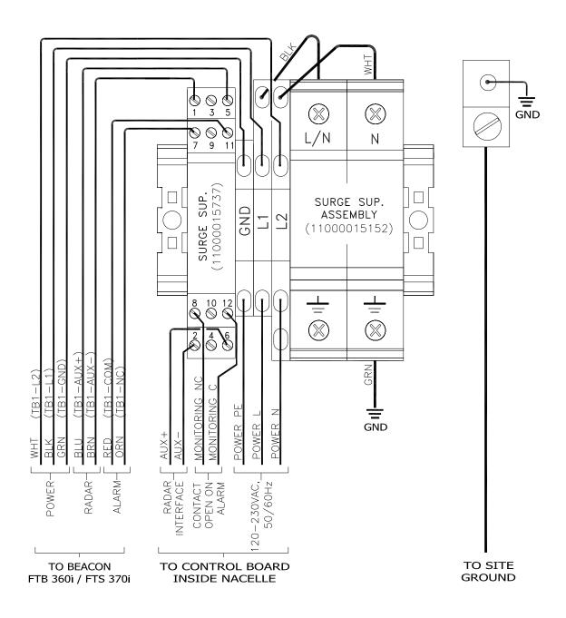
Figure 2-3 – OVP-RADAR Internal Wiring
