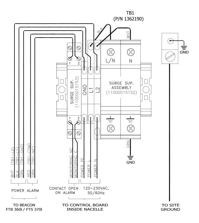
Figure 2-1 – OVP Internal Wiring
