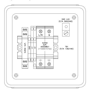
Figure 4-1 – OVP Component Locations
