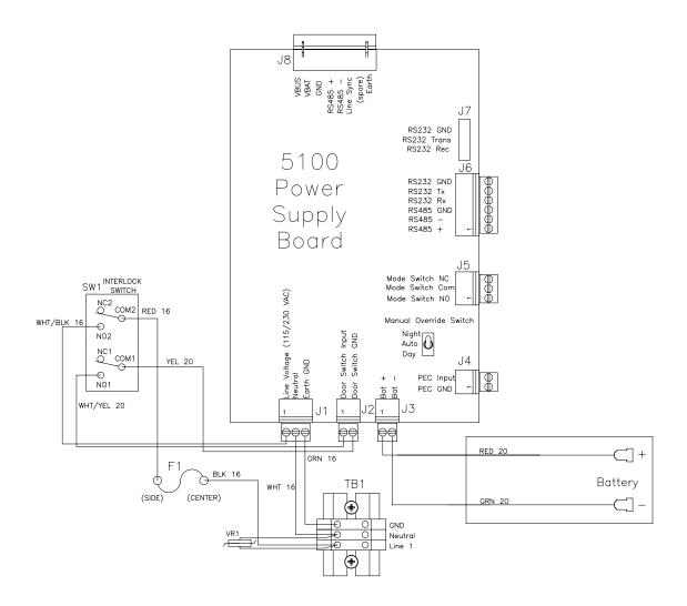
Figure 2-2 FTM 5009 Wiring Schematic
