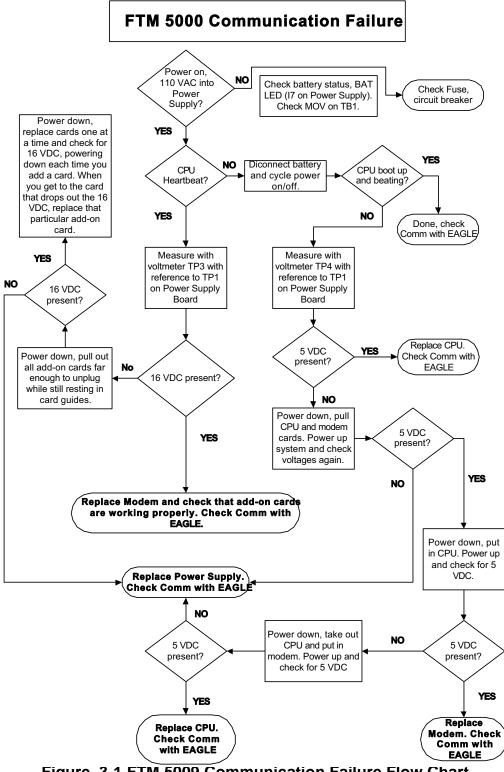
Figure 3-1 FTM 5009 Communication Failure Flow Chart
