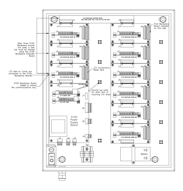
Figure 1-6 FTM 5009 Assembly Backplane Installation
