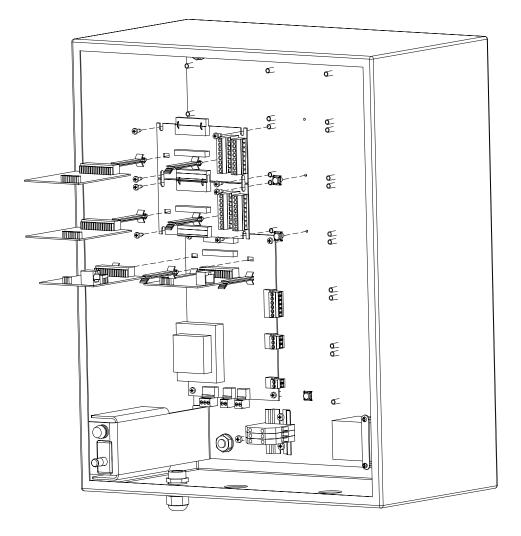
Figure 1-5 FTM 5009 Assembly Showing Optional Add-on Cards
