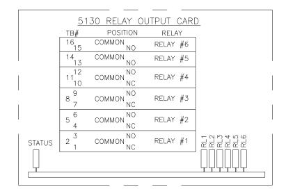
Figure E-1 5130 Relay Output Card Terminal Block Labels
