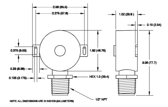
Figure B-3 Photocell Sensor Mounting and Outline
