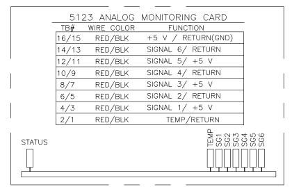
Figure F-1 5123 Analog Input Card Terminal Block Labels
