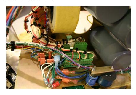
**Step 5**Attach the other end of the cable harness to TB1 and to J4 of PCB1. The exact locations are listed below. The harness has been crimped with the wires in the correct order to simplify installation.
