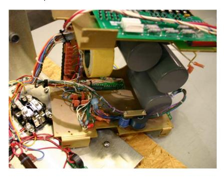
**Step 3** Install PCB5 with the included hardware.
