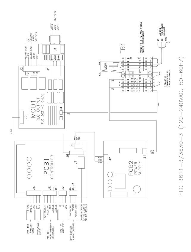
Figure 2-22 - Controller Internal Wiring
