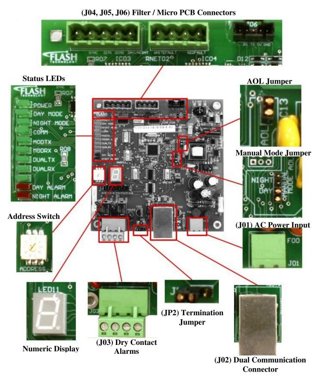
Figure 1-5 - PCB1 Dual Interface Board
