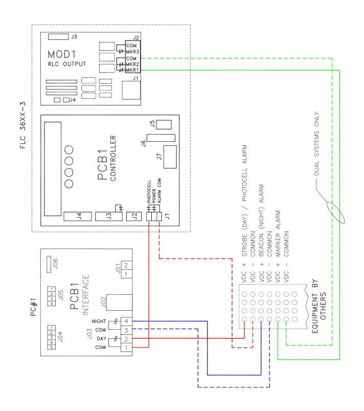
Figure 2-19 - E1 & D1 Dry Contact Alarms For Equipment By Others
