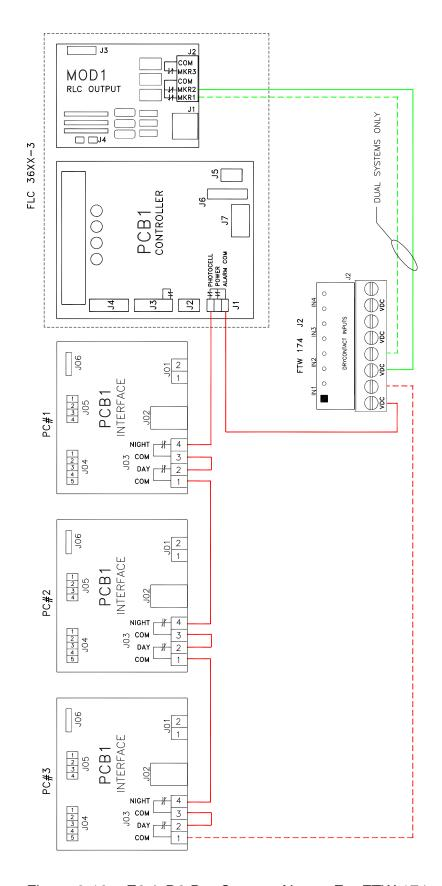
Figure 2-18 – E2 & D2 Dry Contact Alarms For FTW 174
