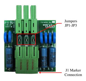
Figure 1-4 – PCB MOD1 Red Light Output Board
