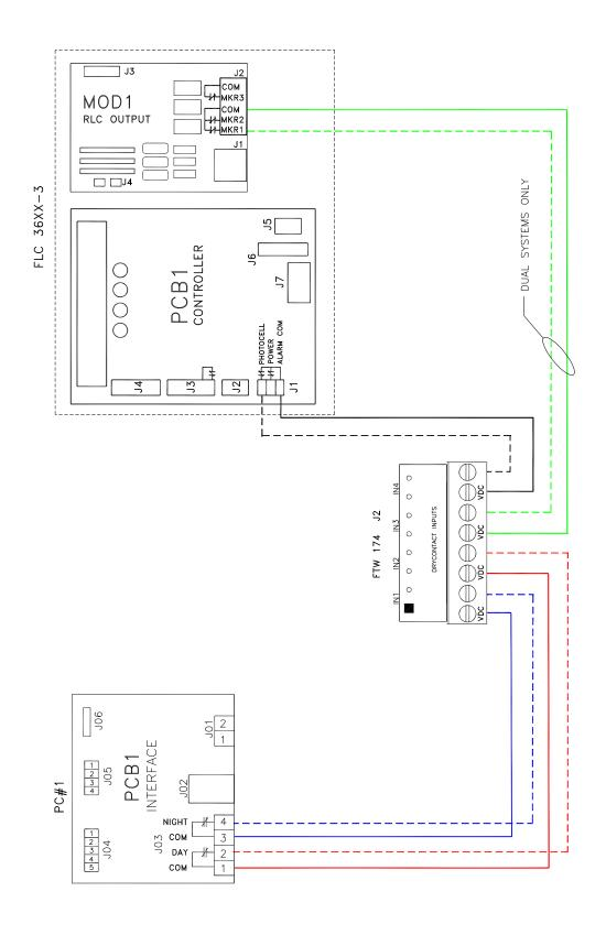
Figure 2-17 – E1 & D1 Dry Contact Alarms For FTW 174
