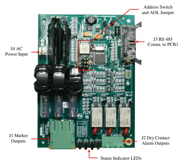
Figure 1-3 – PCB MOD1 Red Light Output Board
