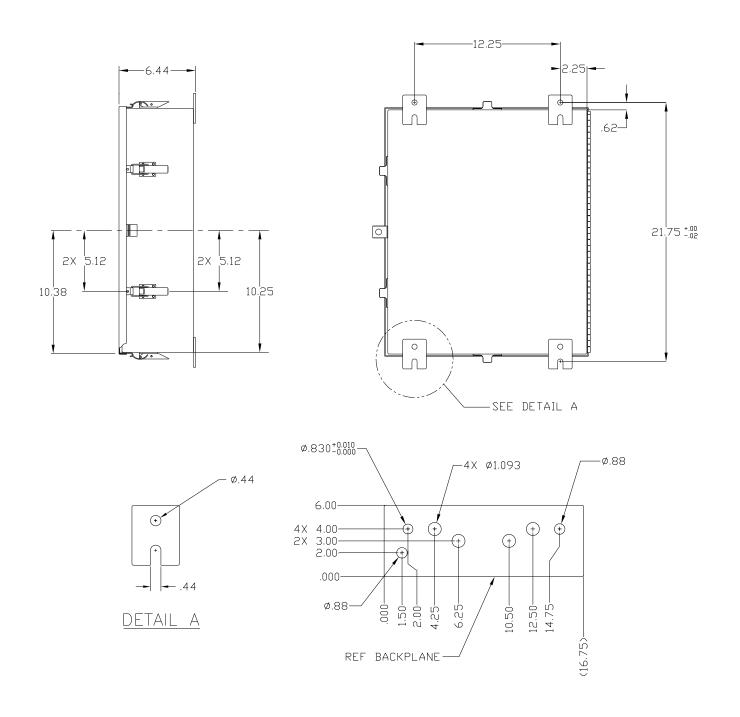
Figure 2-9 – Power Converter Mounting and Outline
