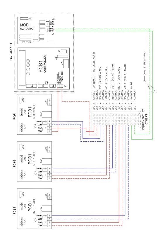
Figure 2-20 - E2 & D2 Individual Dry Contact Alarms For Equipment By Others
