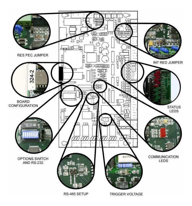
Figure 1-2 – 2903800 Board Configuration
