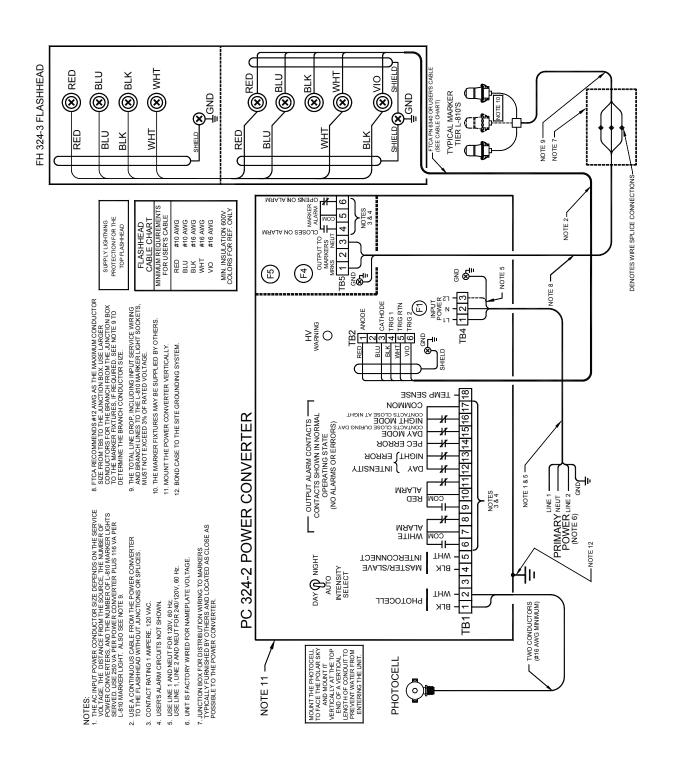
Figure 2-4 – Typical System Installation
