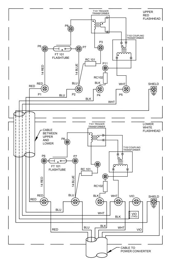
Figure 2-9 - FH 324 Internal Wiring
