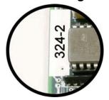
The 2903800 board is programmed from the manufacturer for operation in the PC 324. The board will be clearly marked in the area shown in Figure 1-2.
