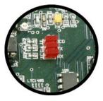
The TX and RX LED's indicate the transmission and reception of data through the board's serial port via the RS-232, RS-485 or the modem card. The DCD LED will be active when a connection has been made via the modem.
