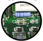
The trigger voltage neon provides an indication that trigger power is being supplied to the 2903800.
