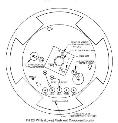
Figure 4-2 – Flashhead Component Layout
