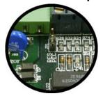
The RES PEC jumper is removed by default. The FTB 324 uses a PEC 510 resistive photocell for determining mode transition. To use an AC photocell, short this jumper and connect the output of the photocell to pins 4 (AC) and 5 (Return) of J5.
