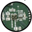
RS485TERM and RS485PUP are open by default and should be shorted only on the last 2903800 board in the series of equipment connected to an FTM-5000 or an FTW 17X series monitoring unit.
