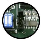
The RS-232 port allows programming and troubleshooting using Tech Eagle shown below (available for download from <a href="https://www.flashtechnology.com">www.flashtechnology.com</a>):
