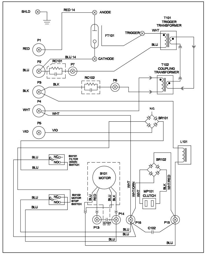
Figure 2-9 FH 306 Flashhead Internal Wiring
