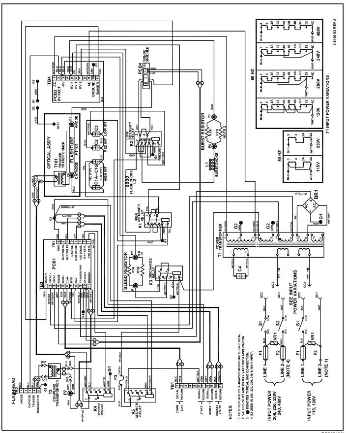
Figure 2-13 FTB 225-1 Beacon Internal Wiring
