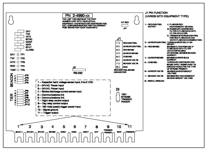
Figure 1-2 PCB1 Timing and Trigger Board
