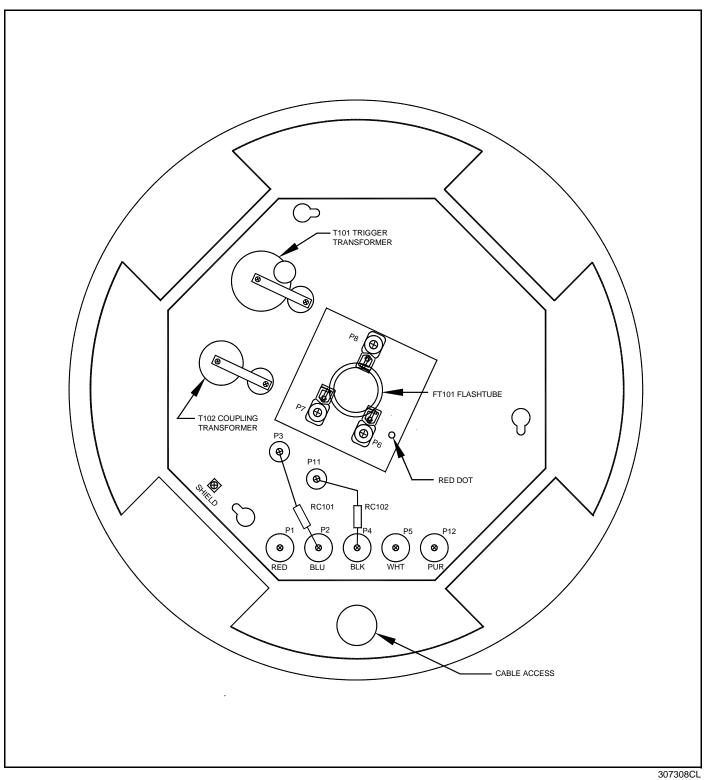
Figure 4-7 FH 307 Flashhead Component Locations
