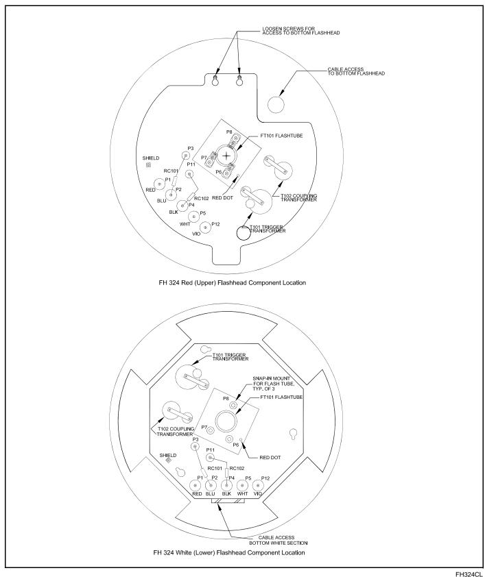
Figure 4-8 FH 324 Flashhead Component Locations
