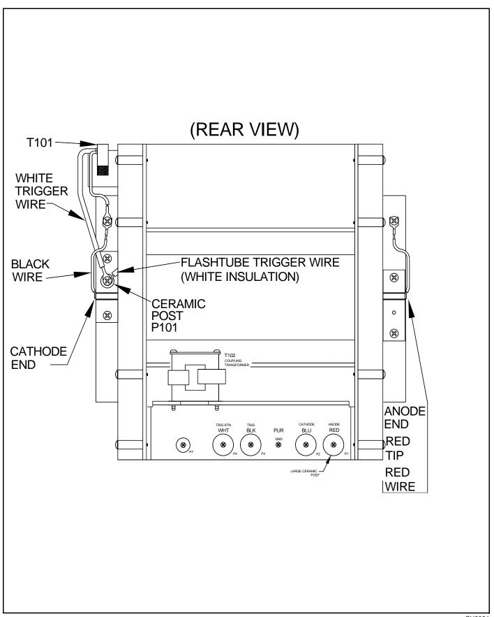
Figure 4-4 FH 204 Flashhead Component Locations
