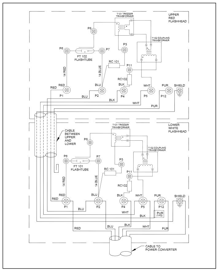
Figure 2-8 FH 324 Flashhead Internal Wiring
