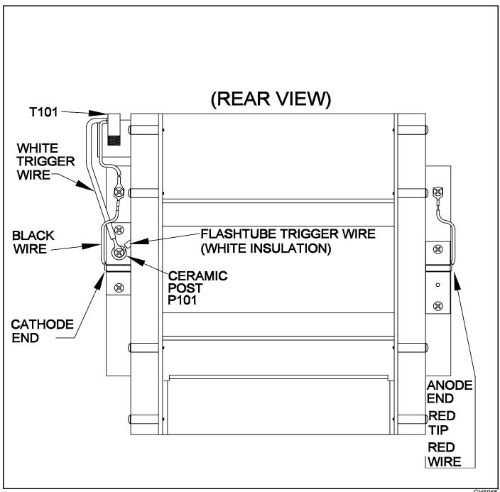
Figure 4-5 FTB 225-1 Optical Assembly Component Locations
