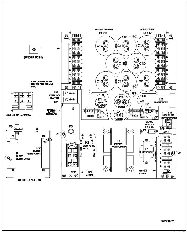
Figure 4-2 PC 224-1 Power Converter Component Locations
