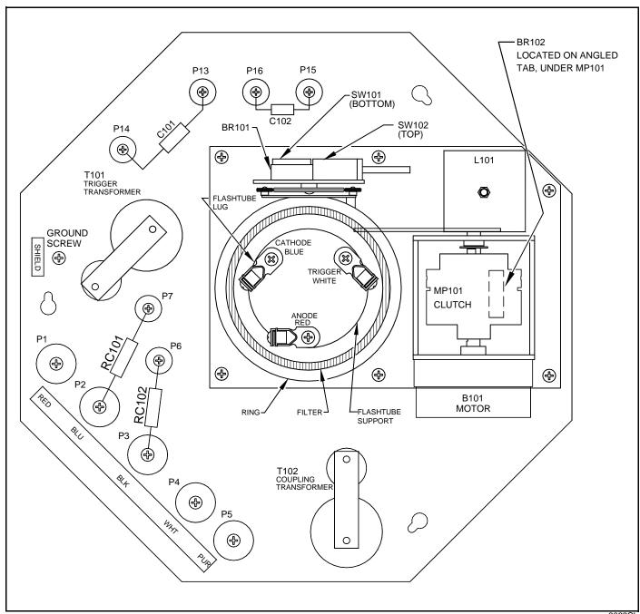
Figure 4-6 FH 306 Flashhead Component Locations
