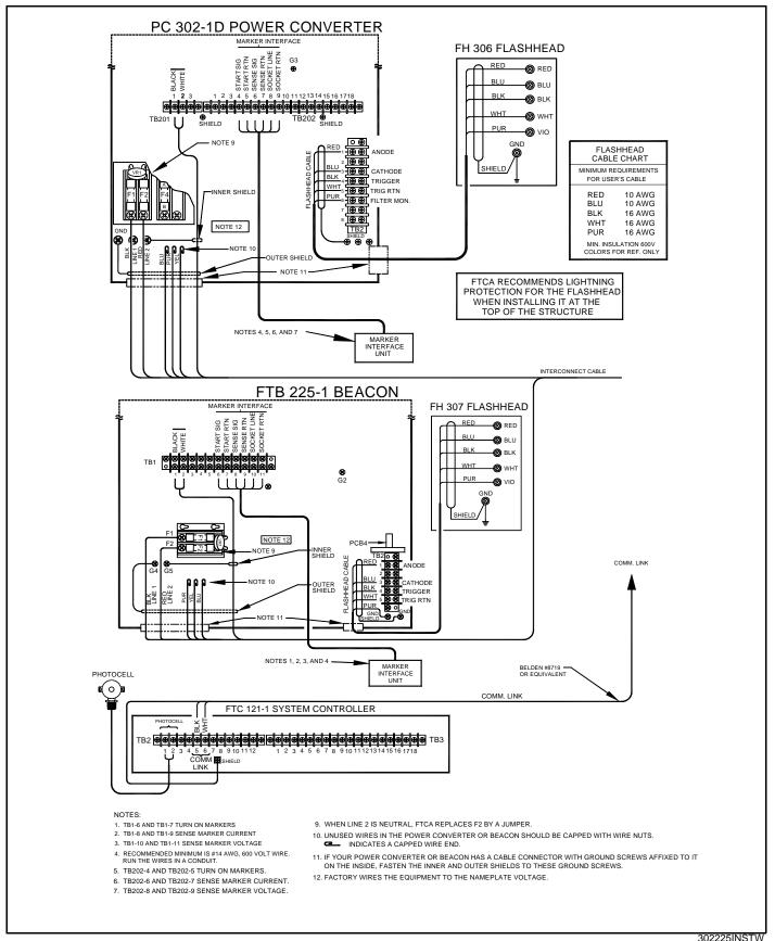
Figure 2-18 FTB 302-1D and FTB 225-1 Installation Wiring Guideline
