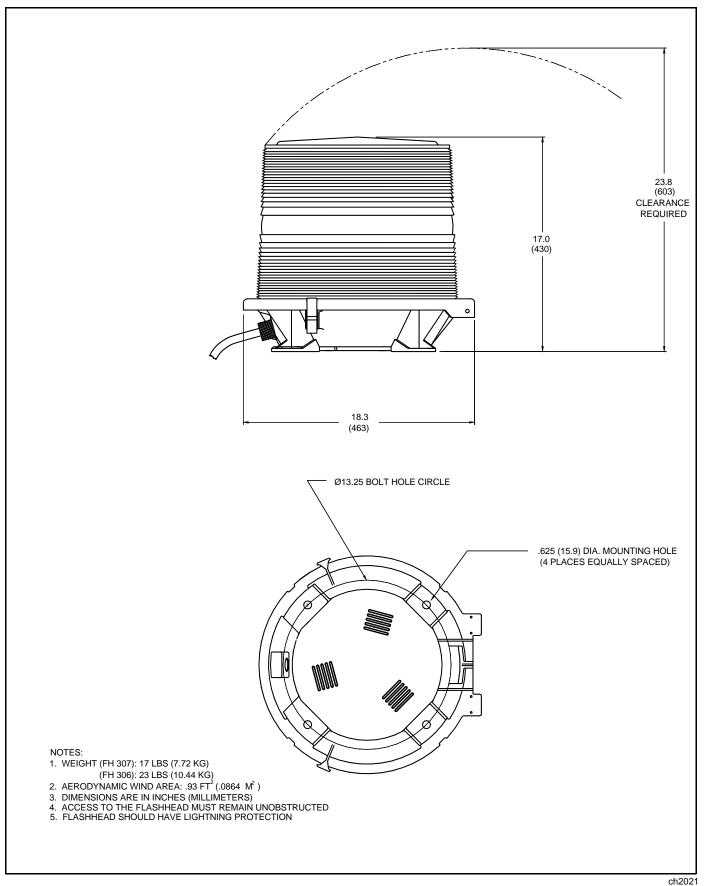
Figure 2-4 FH 306 and FH 307 Flashhead Mounting and Outline
