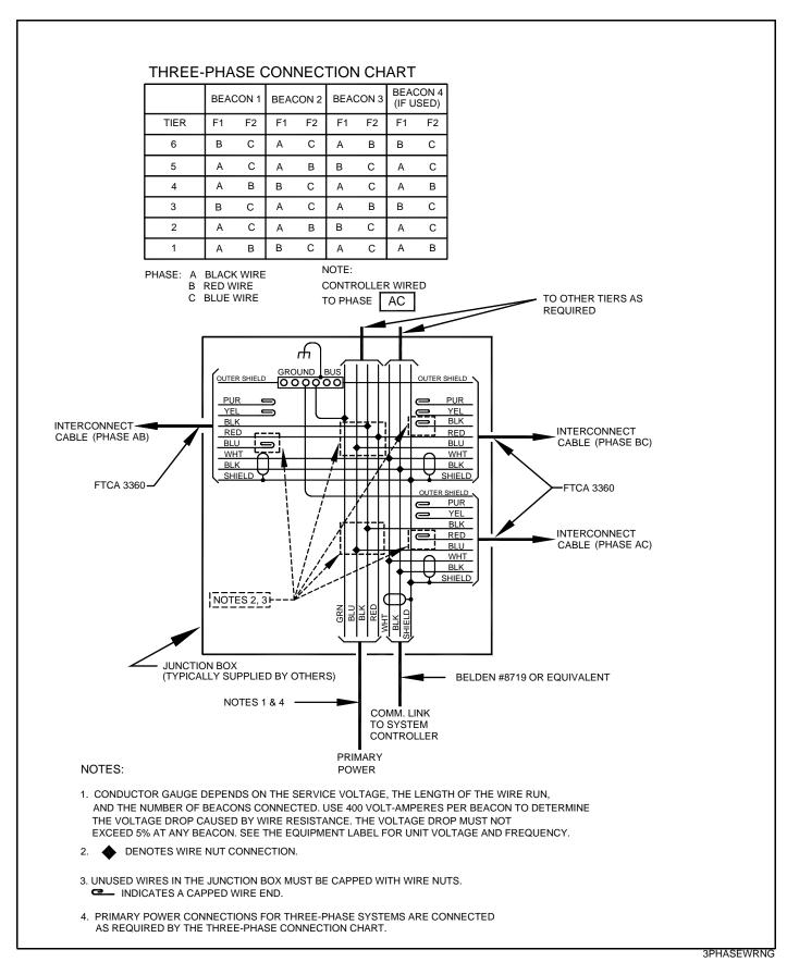
Figure 2-16 Junction Box; Three-Phase Wiring Guideline
