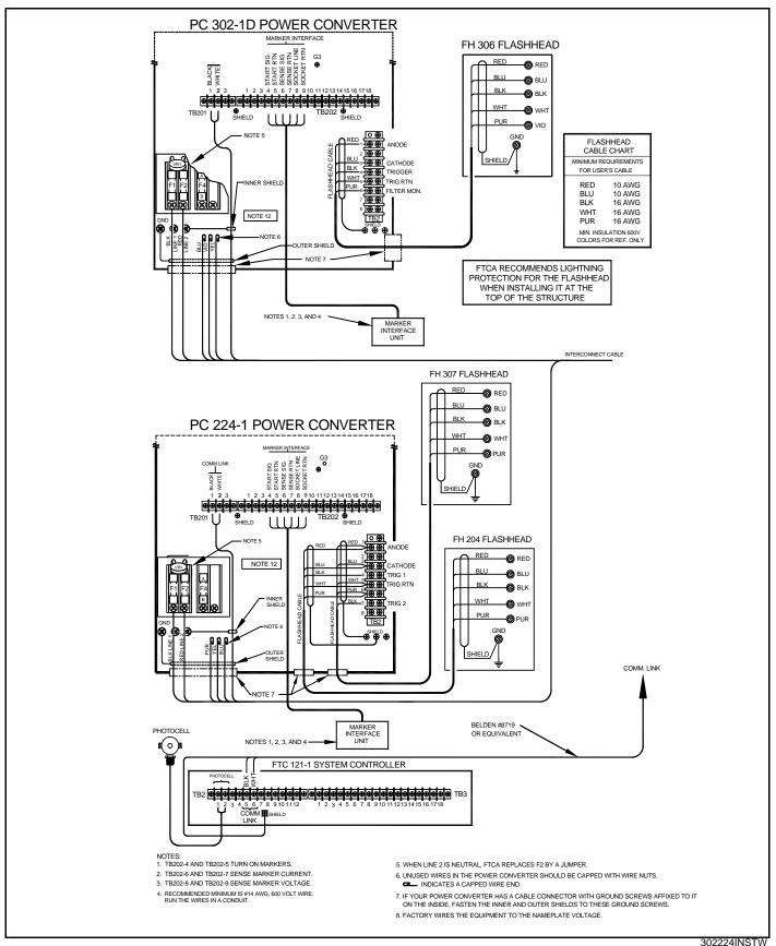
Figure 2-17 FTB 302-1D and FTB 224-1 Installation Wiring Guideline
