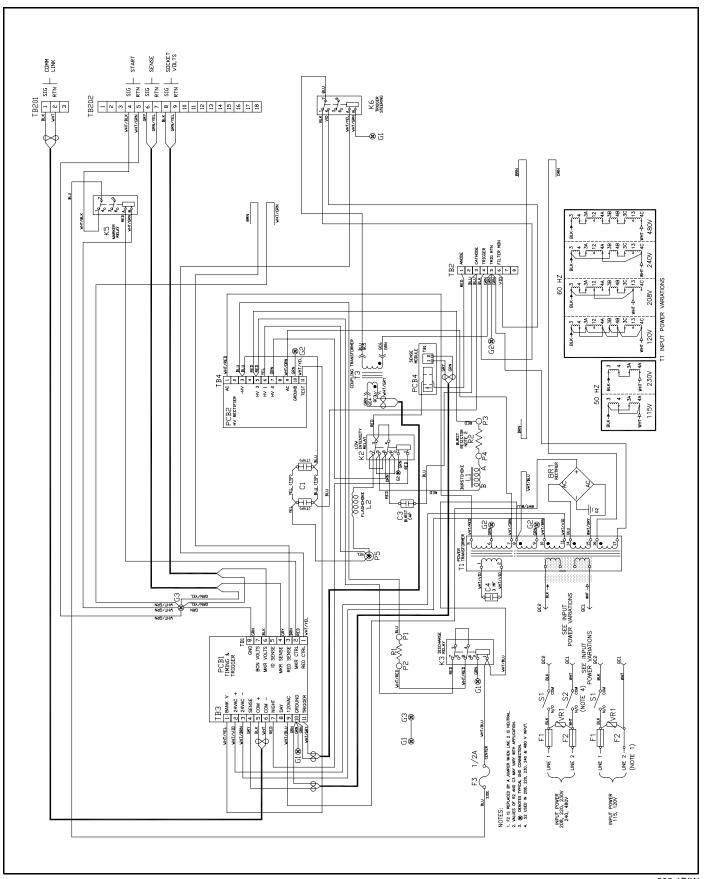
Figure 2-11 PC 302-1 Power Converter Internal Wiring (FH 324)
