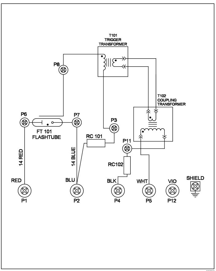
Figure 2-7 FH 307 Flashhead Internal Wiring
