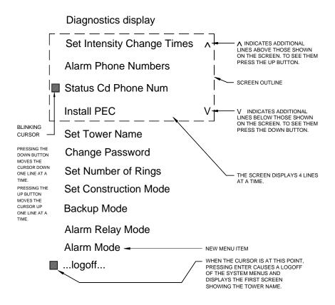
The Alarm Mode screen allows you to select the operation of the main alarm relay.
